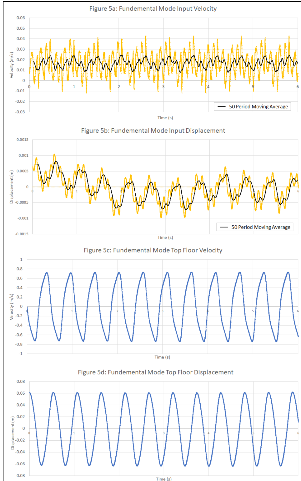
Figure 5: Example of the velocity and displacement time histories—recorded at the fundamental mode of the model structure with the motor and cam system as the driving device. Input velocity and displacement are very noisy, but the top floor velocity and displacement appear to be much cleaner sinusoidal responses. Fifty period moving averages demonstrate the periodic nature of input excitation.
