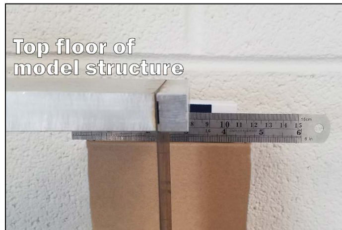
Figure 3: A ruler positioned behind the top floor determined maximum displacement during excitation. This displacement was then used to manually calculate the velocity transducer conversion rate.
